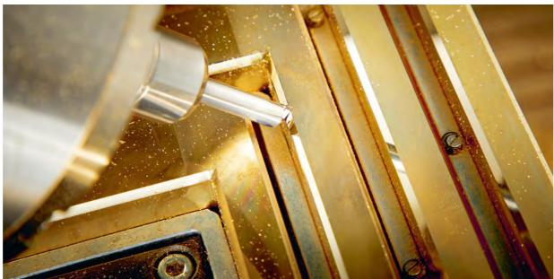
RIGHT: A line that will become a diamond cut in the finished appearance is milled up to five times.
